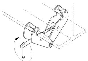
above. Installation is by rotating the handle, of the reverse threaded cross shaft, until the
